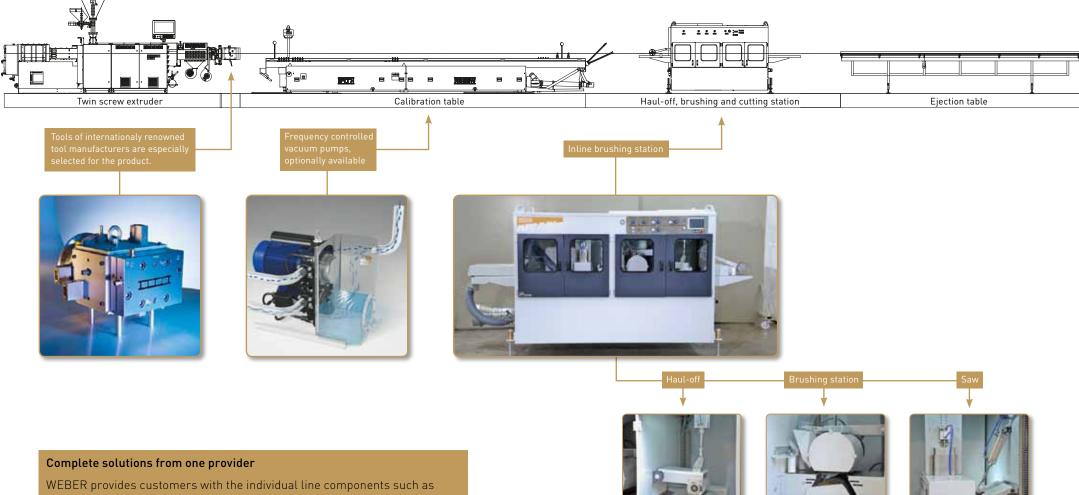
extruders, calibration tables, haul-off, brushing and cutting stations as well as ejector tables, all from one source. This creates an ideal system solution without interface problems – and everything in the usual WEBER quality.
