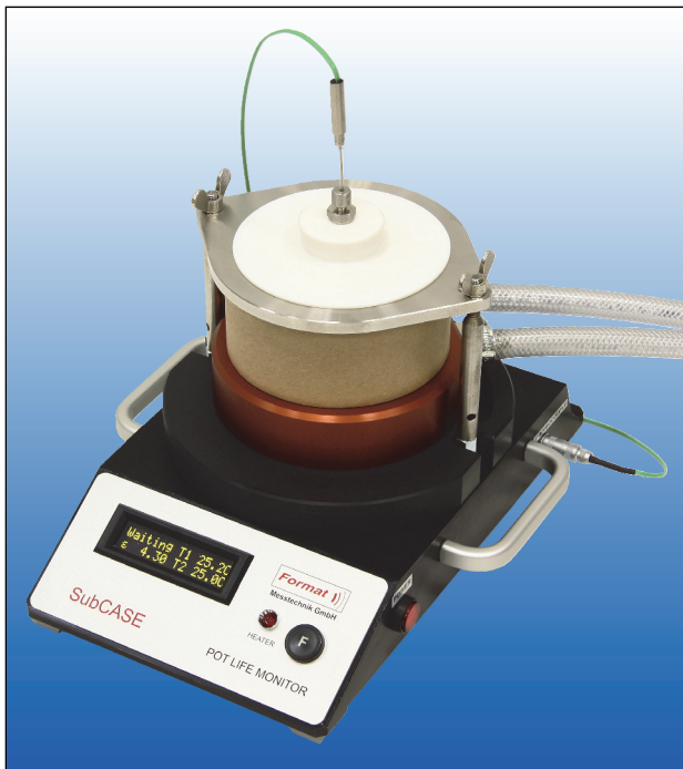
Figure 1: The SubCASE® LT is designed to measure the gelling and curing reaction at low and constant temperatures. The relative permittivity of a formulation can be measured simultaneously at different electric frequencies.
