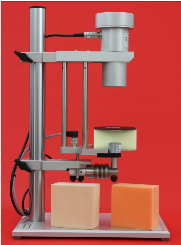
Figure 2: Mechanical setup of Resimat 100 for measuring viscoelastic foam samples of typical 100 \times 100 \times 50 \text{ mm}^3 .
