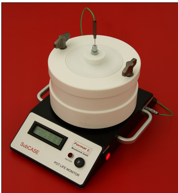
Figure 1: The Test device SubCASE HT* can measure the pot life and the curing of reactive plastics. It is designed for high reaction temperatures. The core temperature is measured by a reusable thermocouple inserted vertically into the center of the plastic sample.
